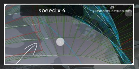
Do you see the scan-surface lattice lines? They don't overlap. You can push in Hulls and at the same time, observe the edge-surface distance
